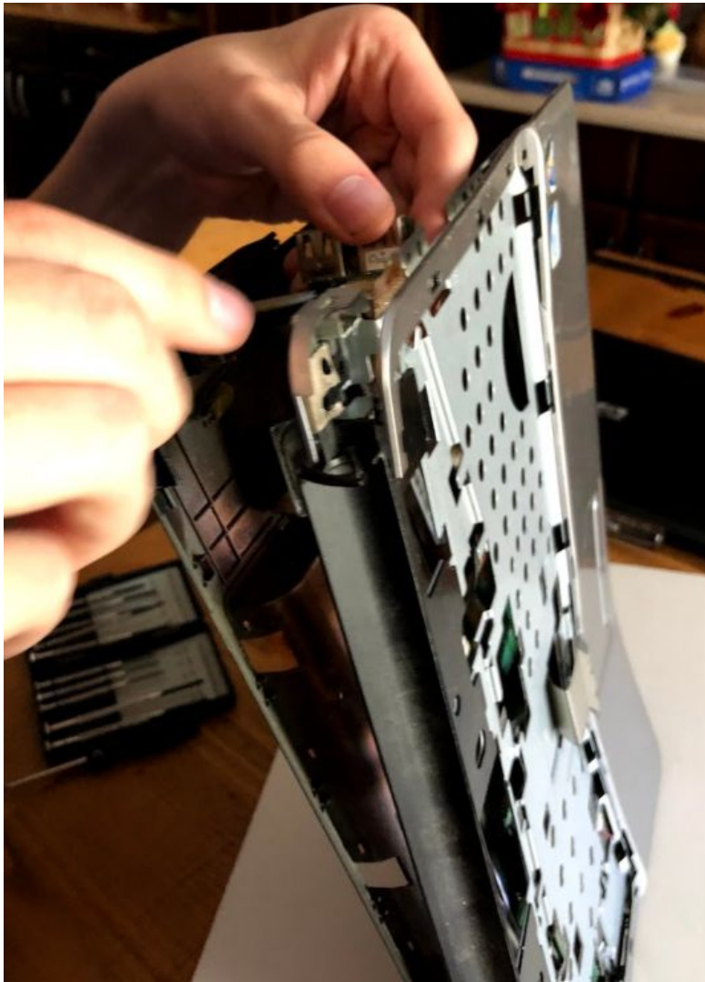
Figure 1.15: Pulling apart the bottom and top plates to expose the internal workings of the computer.
