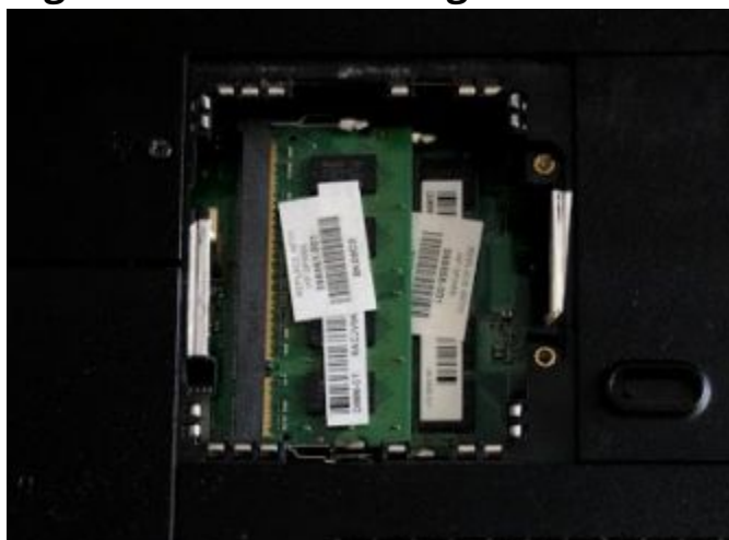
Figure 1.5: Plastic casing removed to show RAM sticks.
