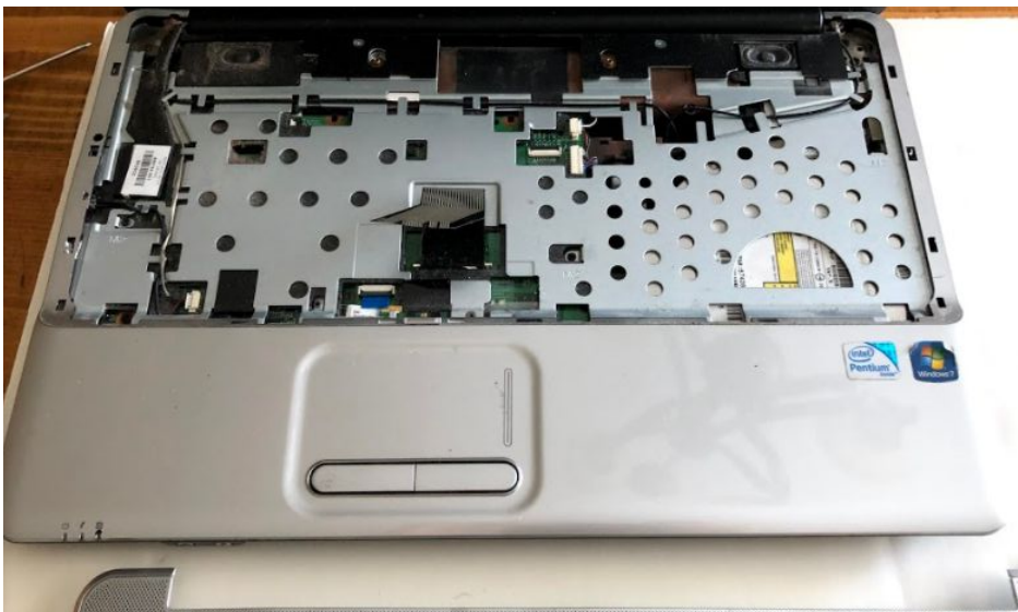
Figure 1.14: Interior laptop view without the top plates present.
