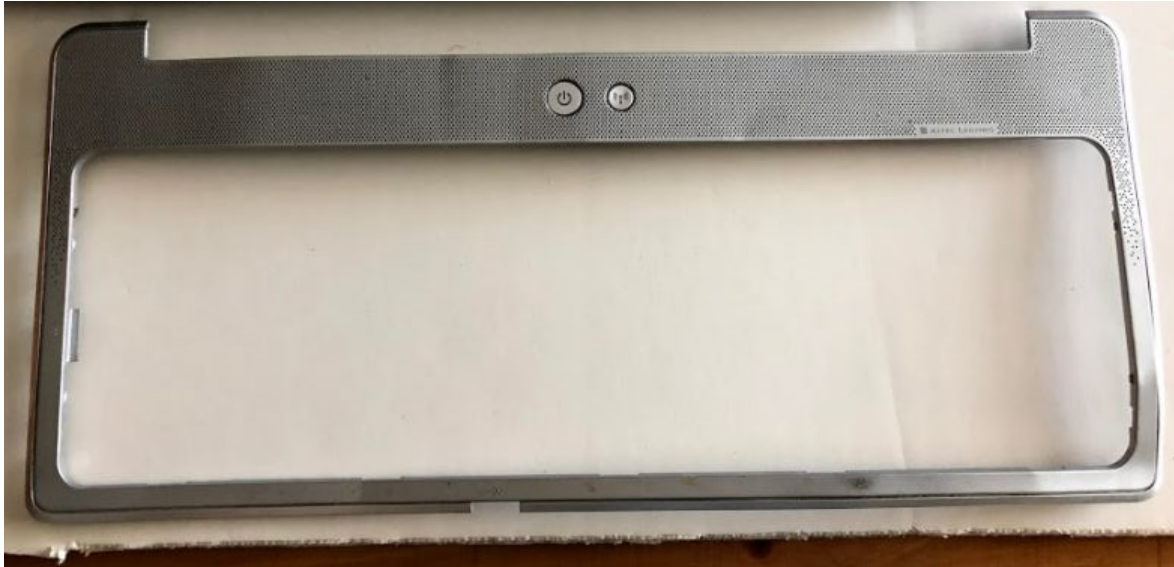
Figure 1.13: Removing the top plastic plate, including power buttons.
