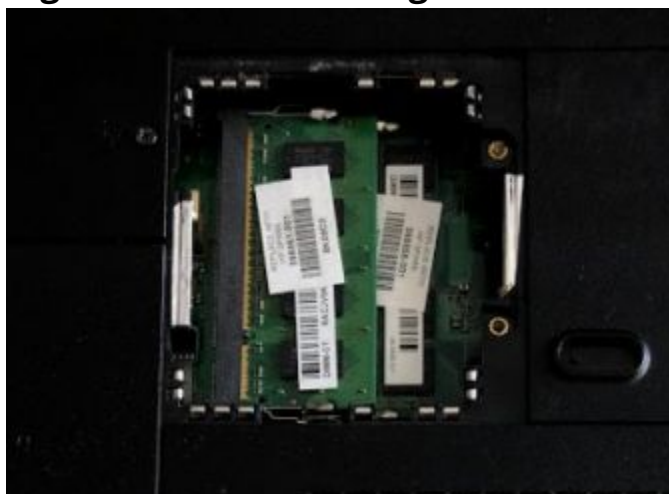
Figure 1.5: Plastic casing removed to show RAM sticks.
