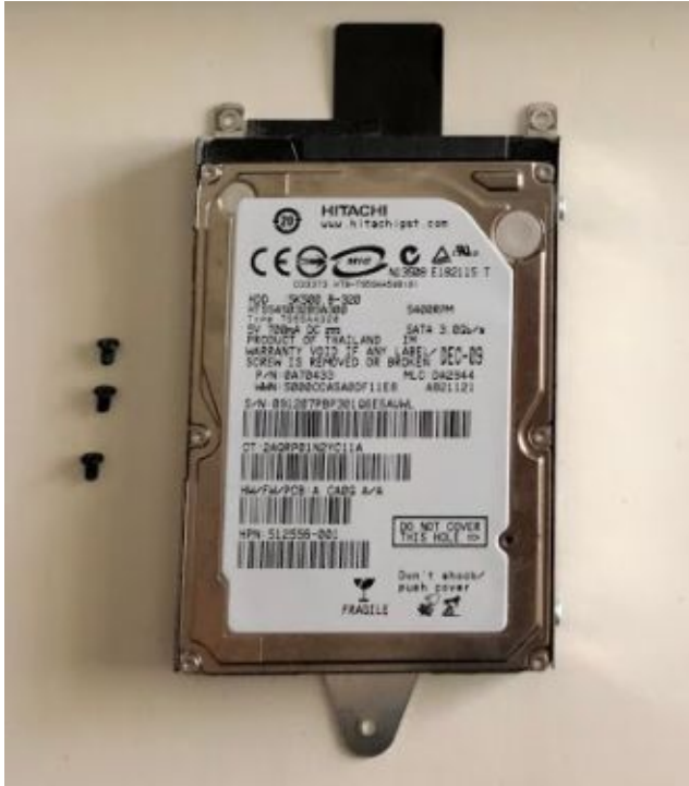
Figure 1.10: Hard drive removed, with screws holding it in place.
