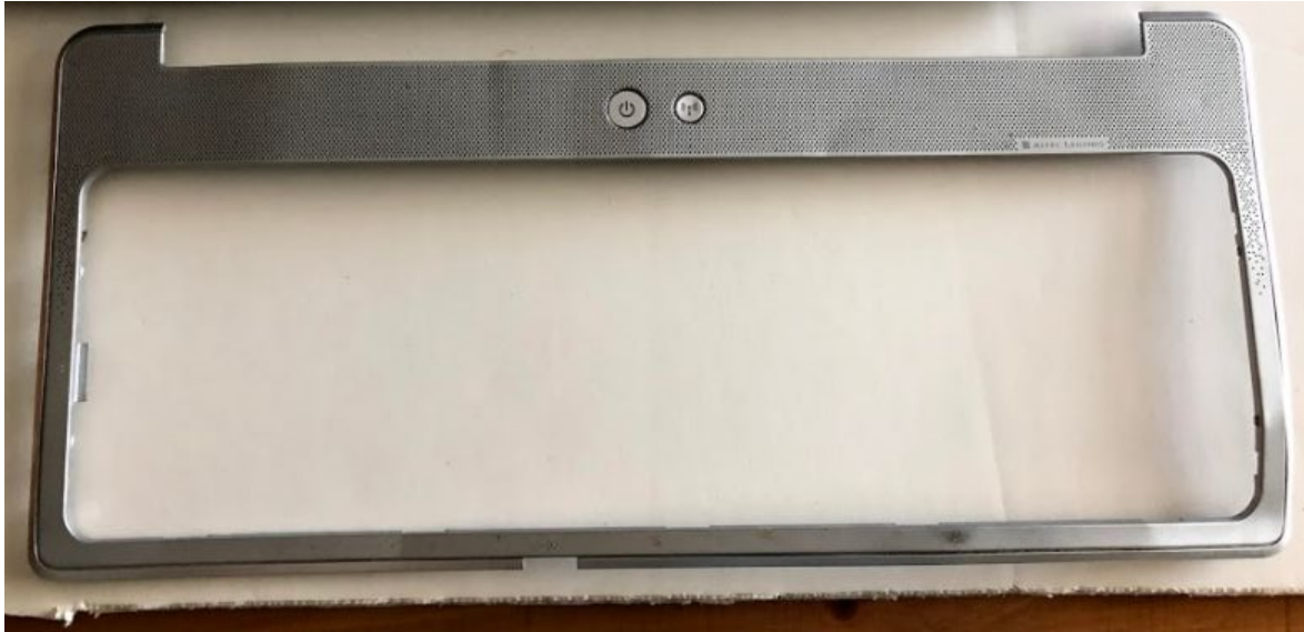
Figure 1.13: Removing the top plastic plate, including power buttons.
