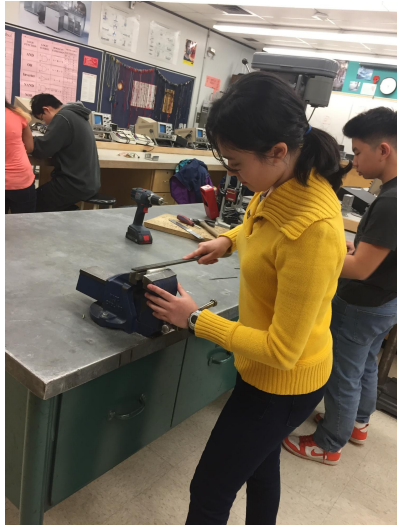
One of our team members, Anaïs, sanding down a 3D printed counterweight prototype
