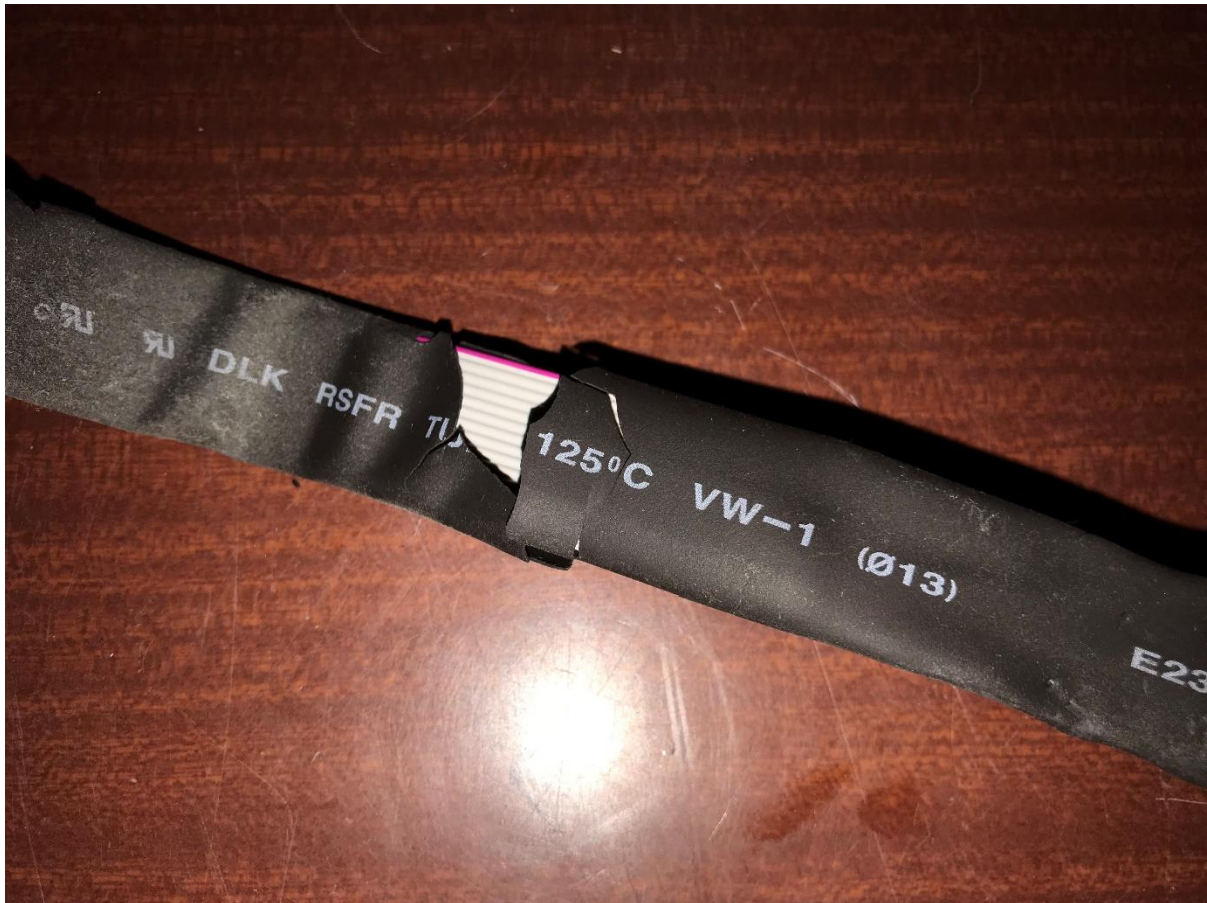
Step 14: Interconnect cable with protective sleeve rated at 125°C brittle and cracking
