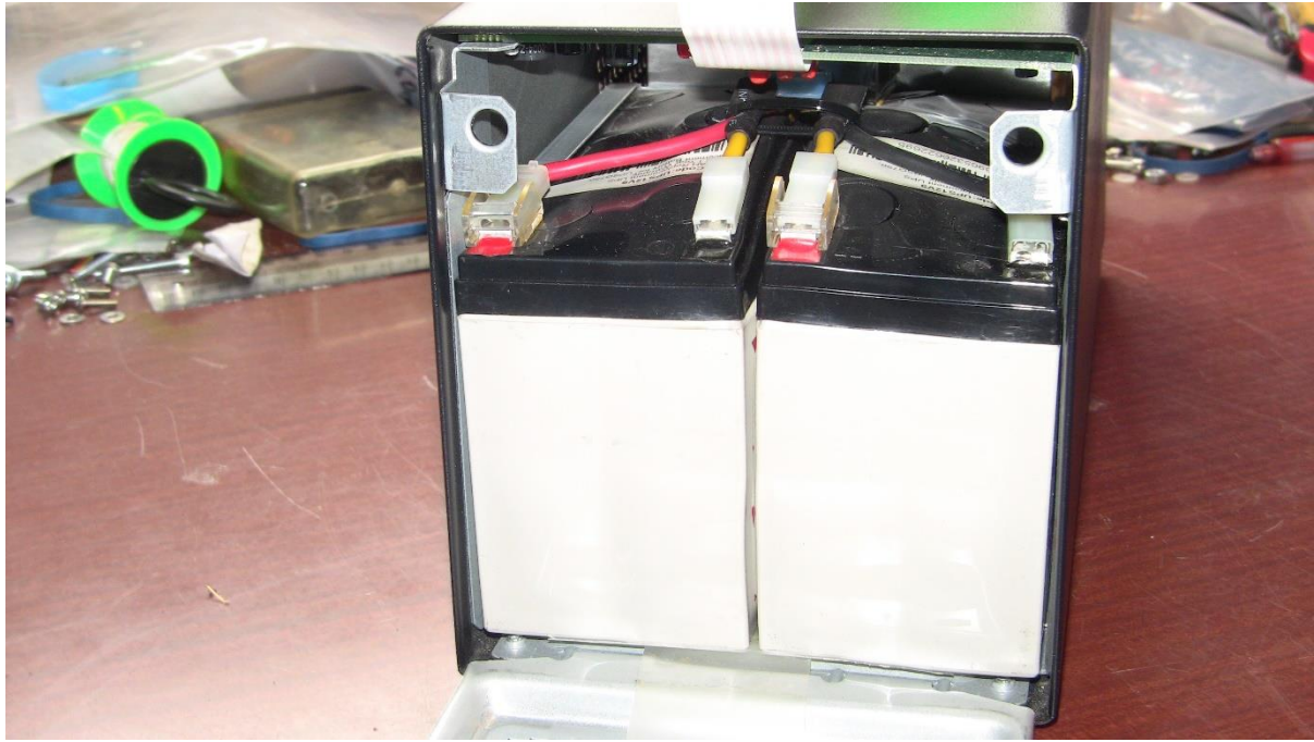
Step 6: Attempt to remove battery pack failed. Noted bulging top and sides.
