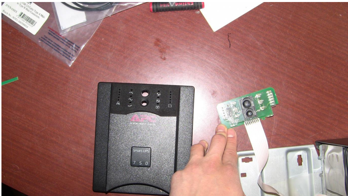
Step 3: Front panel controls board connected by flexible ribbon cable
