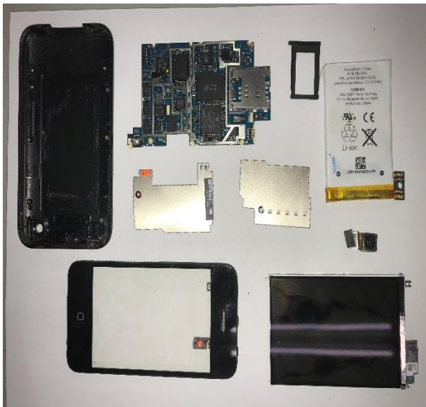
The phone with it's screen pried off and the internal components exposed.
