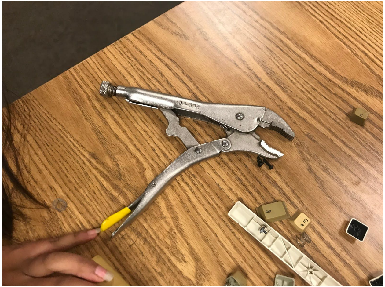
Using a vice grip we were able to take the keys off easily.
