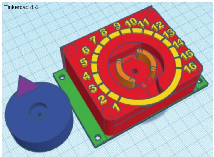
to make space for the rubber shaft collar (Blue). To finish off the knob, I used a triangular prism and a wedge for the pointer (Purple). I then positioned my objects for printing and saved them. Because I already had my measurements and design planned out, as well as the simplicity and user-friendliness of Tinkercad, designing the Autonomous Selection Knob took only about 5 hours to do, over the course of 3 days.
