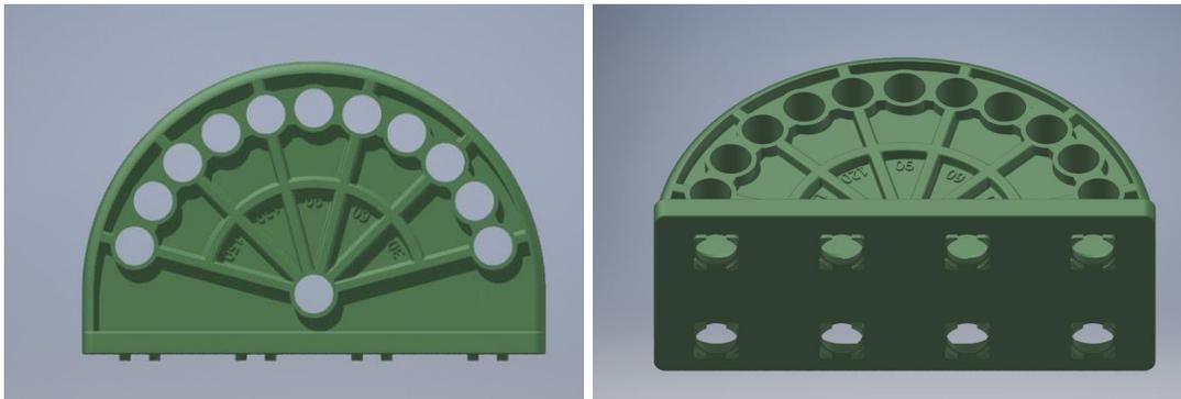
The primary axis “base” piece provides 8 mounting holes to allow teams to easily attach the component almost anywhere on their robots. Each of these mounting holes also features inserts, similar to those in VEX Bearing Flats, for proper alignment to the square holes. The base piece offers 11 slots to secure the Vision Sensor at an angle of 15°-165°, in 15° increments.
