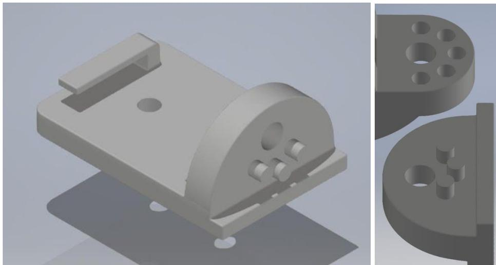
The final camera attachment “plate” piece screws into the back of the Vision Sensor. The plate has 3 small extrusions that can be aligned with the 5 divots on the middle piece to aim ‘left’, ‘right’, and ‘center’ on the secondary axis. The plate also includes a wire management clip to secure the Vision Sensor wire.
