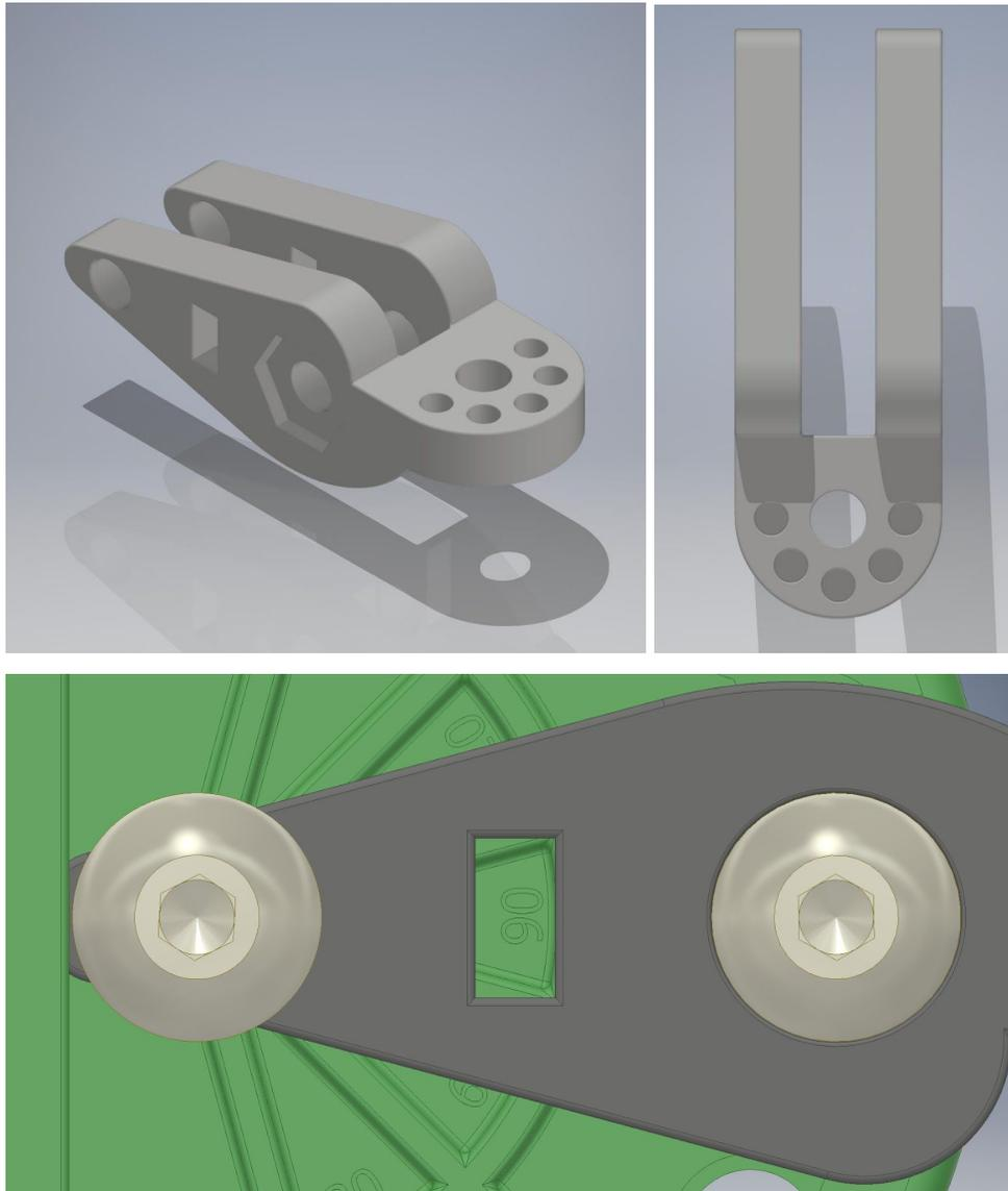
The secondary axis “middle” piece easily affixes onto the base piece with 2 screws and nylock nuts. During building, the team can easily remove the radial screw to test various angle configurations, and then tighten the screws once a perfect setting is found. Labels embossed on the base piece make it possible to record a specific setting. If an extreme circumstance leads to part breakage, it is easy to recreate the same precise alignment on a different Precision Mount system.
