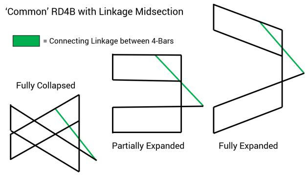
One of the biggest challenges is to make the 2 stages of the lift move in opposing directions. This is often done with a gearing system, however, this has a number of disadvantages, such as:
