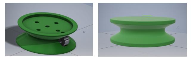
The first iteration was a yoyo-shaped pulley, with a slot for a collar to be inserted to lock onto the string, however, this was soon disregarded. As I got closer to the final design, I 3D printed a prototype, finding issues with the axle bore, and nuts getting in the way of the string. 3D printing allowed me to find these issues quickly, and solve them easily.
