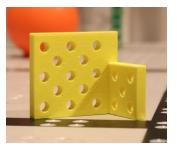
that can attach to a motor, but also attach to any beam. So, we took a ruler, a motor, and over 10 hours of Autodesk Inventor training to make the perfect piece. Our "Smarter Motor Mount" is lighter, simpler, and much much better than any other mounting method.
