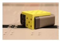
aim to eliminate all issues when mounting a motor, such as drift, friction, and overall complexity. This piece could easily make any existing design more stable, and simpler to repair. Most teams would have to temporarily take apart their entire mounting system for repairs, but if they used this piece all they would have to do is just snap it off.
