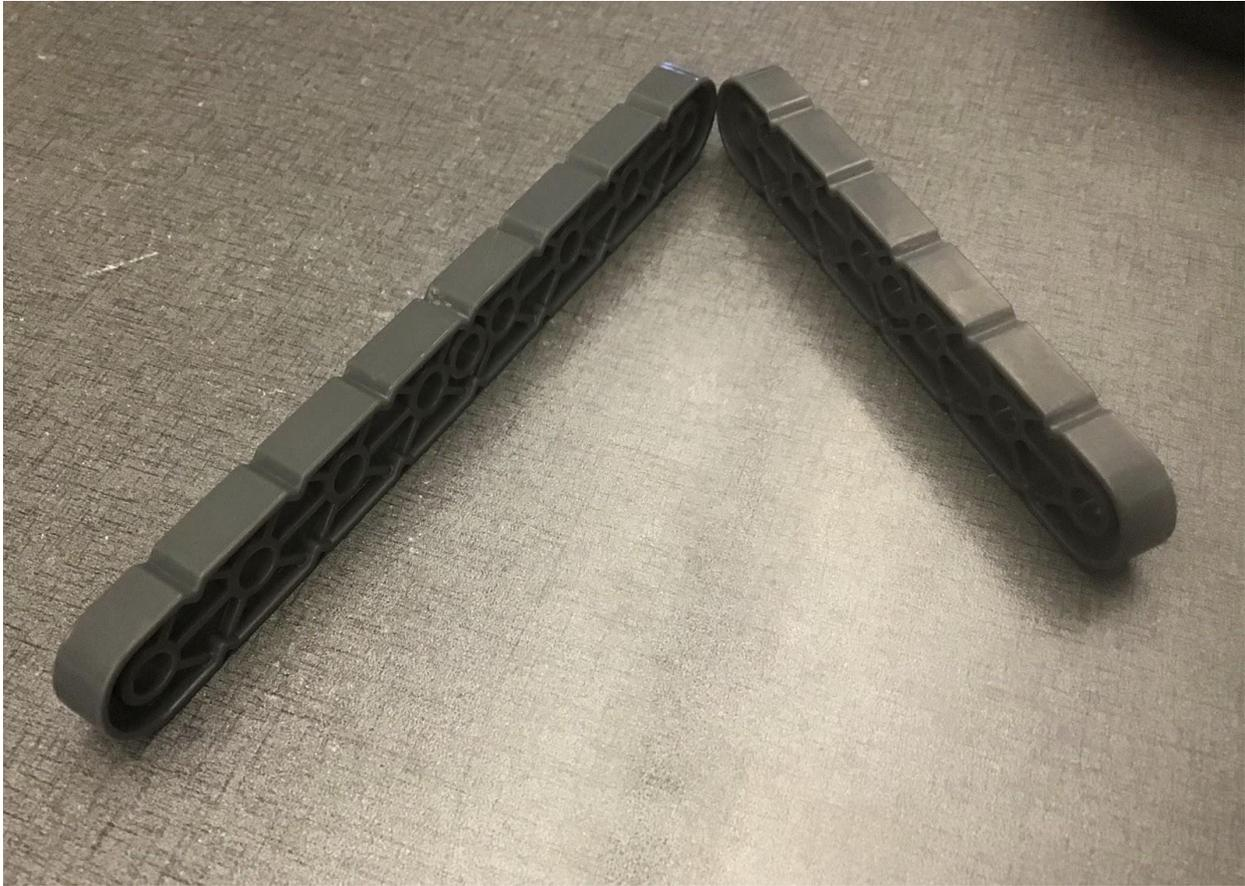
If a robot had parts in the way of putting a corner connector where the two beams must meet, or especially if they needed an angle other than 90 degrees, then our Bent Beam would be used. After all, the part would come in more than the 90 degree angle shown in our design, but we chose to design an example of a 90 degree angled Bent Beam.
