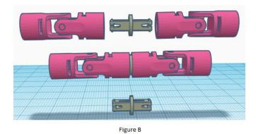
This would allow us to raise and lower the arm without the universal connector locking up.
