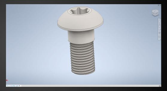
There would be 2 sizes for the lip: 1/8in and 1/16in. Each size would be made between a 32nd-64th of an inch smaller than those measurements to allow the nut to continue to screw into the metal and hold the parts together with a small amount of compression. The reason the screws would be available for both sizes is so that the lip can be used with either one single piece of building material, or two pieces that are flush with each other.
