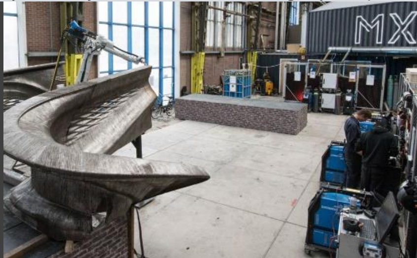
10 MX3D Robot Printing Steel Bridge ( https://www.jorislaarman.com/work/bridge-update/ )
