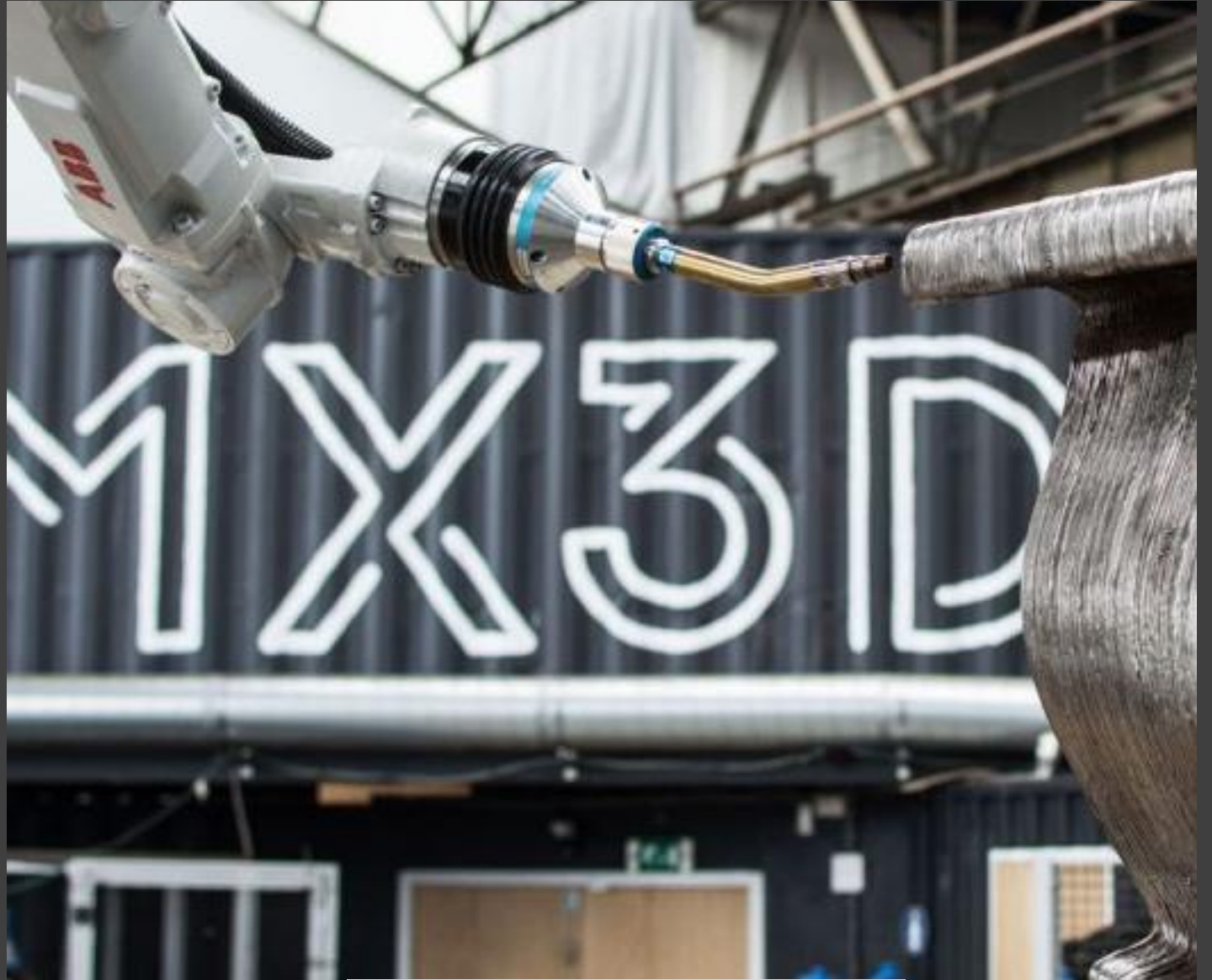
11 The First Tests of the MX3D Robot Printing ( https://mx3d.com/projects/mx3d-bridge )
