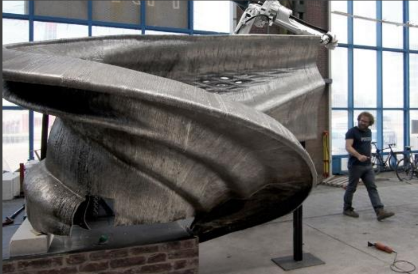
9 MX3D Robot Printing Steel Bridge ( https://www.jorislaarman.com/work/bridge-update/ )
