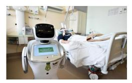
Robots like Tommy are used to measure blood pressure and the oxygen saturation for the patients in the ICU. These two parameters provided a crucial picture of the patients' health conditions, and through the use of robotics, doctors are able attain this information quicker and efficiently.
