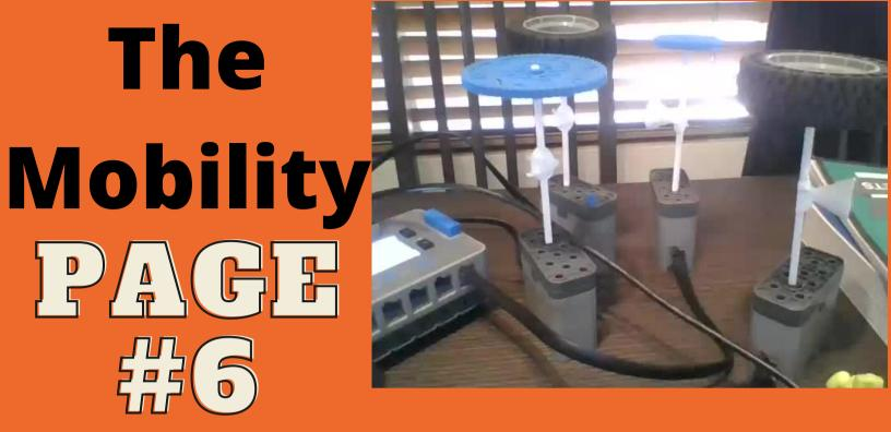
The reason for the magnet on the shaft is to solve the problem that: pieces can go in many ways. So that is why we created the Horivertical Shaft where it can connect multiple pieces together. This magnet was created on the shaft to attach the 2 pieces to make one singular piece that could go horizontal, vertical, or both.
