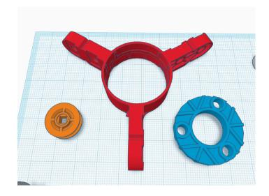
I started modifying the parts and added a 10mm pulley (228-2500-163) because this piece has a square in the middle that a shaft can be locked into to allow the 4-way perpendicular plate to spin or rotate.
