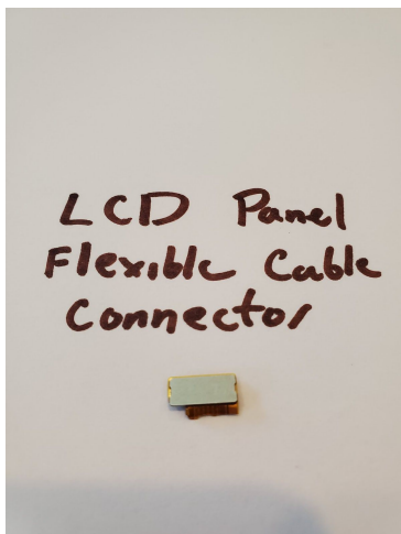
An LCD wire that held the screen to the motherboard.
