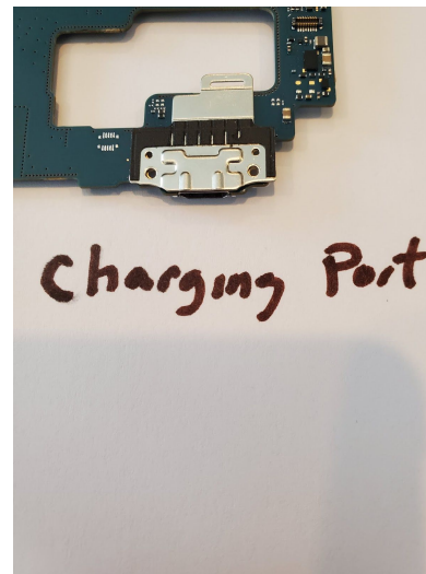
You plug the charger into this then a wire plugs into the battery.
