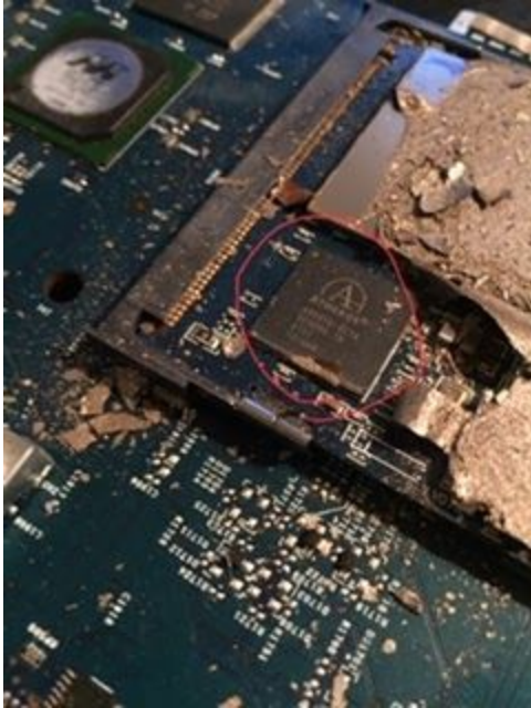
Atheros AR5416-AV1A - Transmits the Wifi signal of 2.4 Ghz and 5 Ghz
