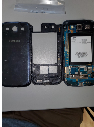
Back plate removed. Circuitry exposed.
