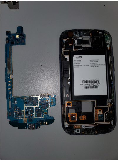
Motherboard removed from phone.
