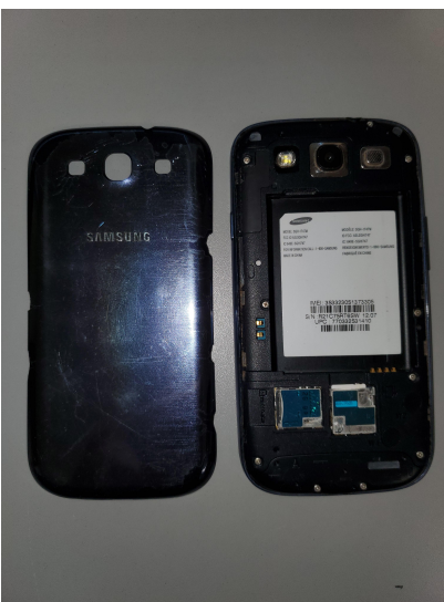
Back cover removed. Absence of battery noted. Phone fully discharged.
