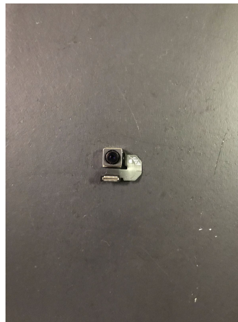
This is the Primary Camera, the device that takes pictures and videos.
