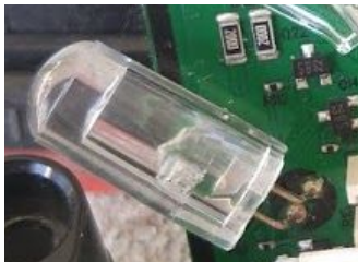
Figure 5.2 Small LED distance sensor (Qty: 2)
