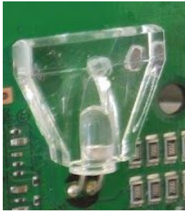
Figure 5.2 Small LED distance sensor (Qty: 2)
