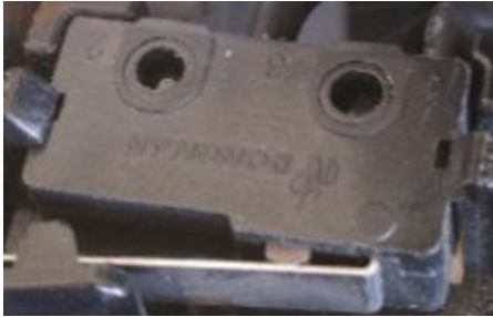
Figure 5.0 Dongnan KW4A(S) Bumper Switch(Qty: 5)
