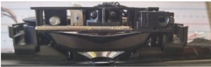
Figure 5.4 Front mapping sensor and cliff sensor (Qty: 5)
