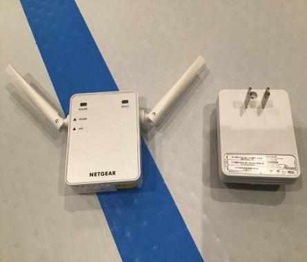
The antennas are used to pick up weak WiFi signals and reproduce them. The housing splits in half in the middle when the screws are removed, revealing the electronic components.
