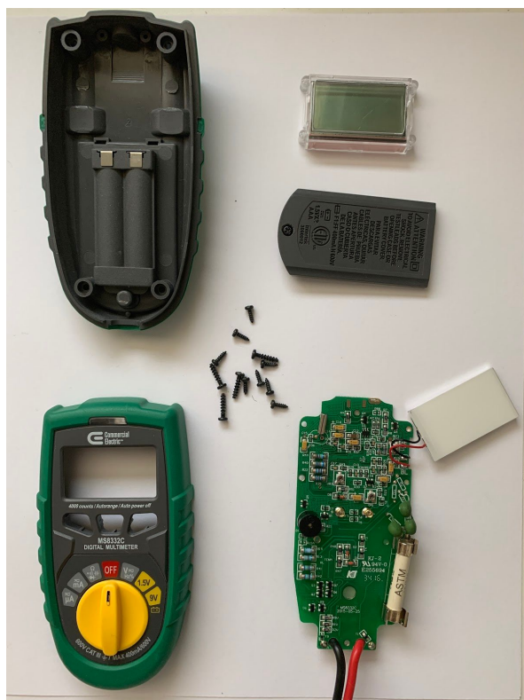
Bottom left: front piece with switch; Top Left: Back Cover; Top Right: LED Display and cover; Bottom Right: Circuit
