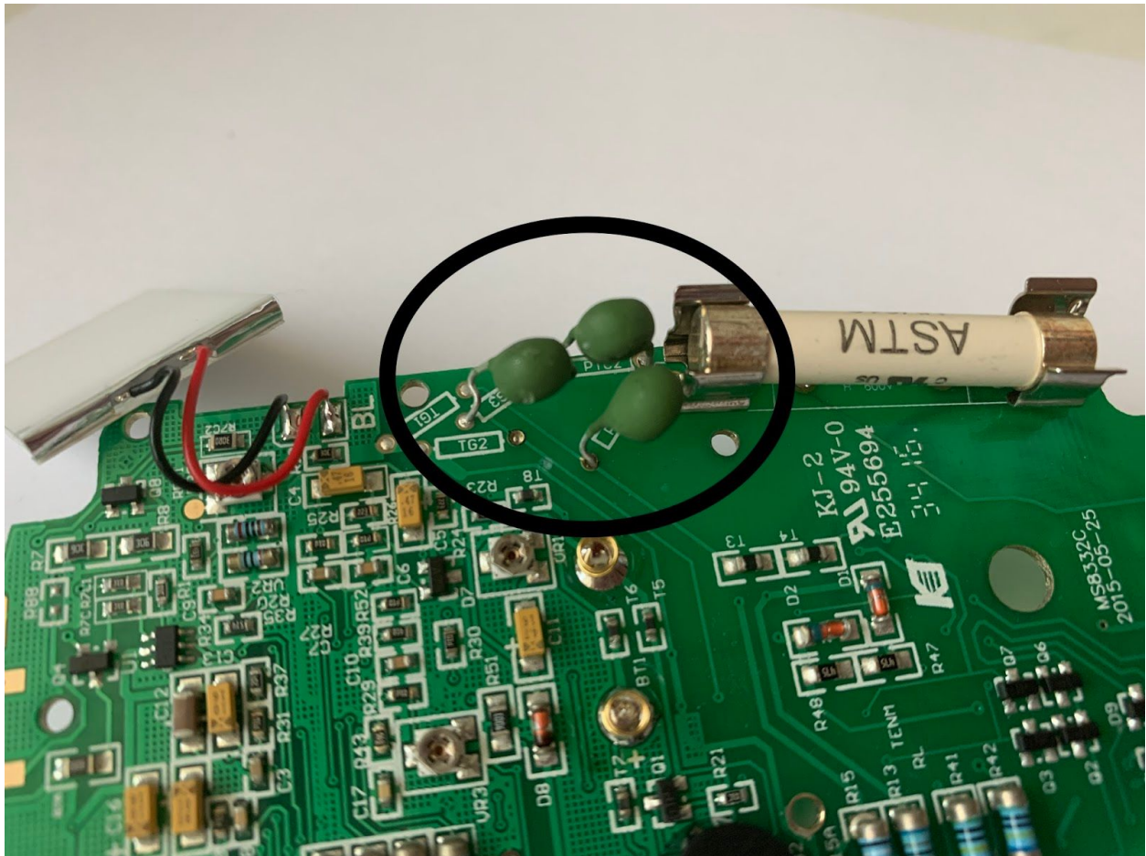
Metal Oxide Varistors; protect the circuit from high voltage spikes
