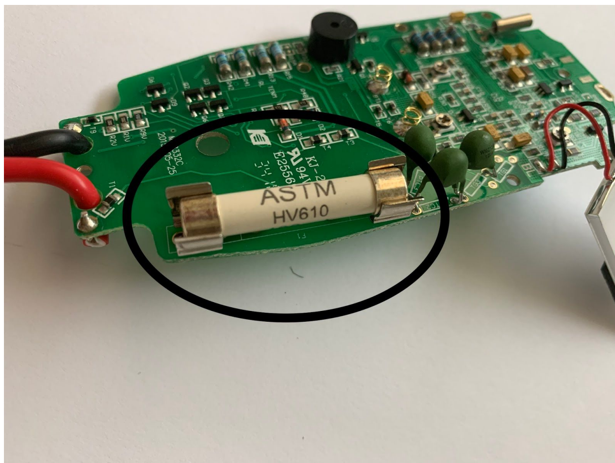
Fuse of the multimeter (HV610); 400mA; Protects the circuit from current overload
