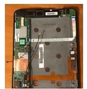
This is the Kindle once the battery was removed. The () and () can be seen clearly here, which connect the camera and headphone jack to the motherboard.
