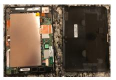
These are the 2 parts of the kindle once the backplate had been removed. The battery, motherboard, and speaker system can be seen clearly here.
