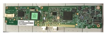
This is the motherboard of the Kindle. The Flash Memory, RAM, CPU, Power Management IC, and GPS are some of the components on the motherboard.
