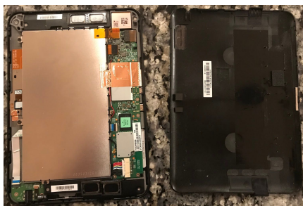
These are the 2 parts of the kindle once the backplate had been removed. The battery, motherboard, and speaker system can be seen clearly here.
