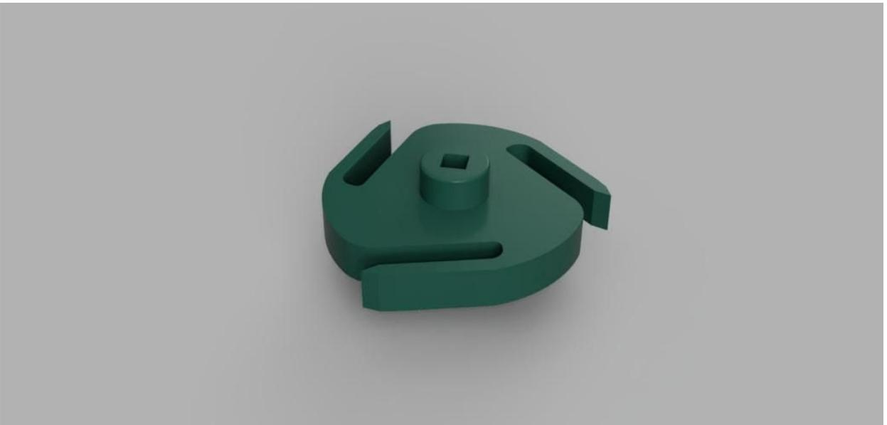
The way the rotor sits in the outer base has been improved over time so it can withstand more load when the sprocket isn't ratcheting. This is how the rotor sits in the outer base in the final design:
