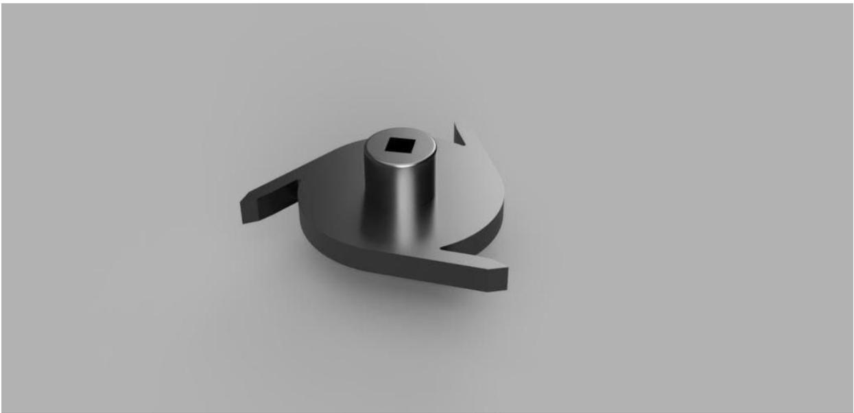
To simplify the design, the same tooth that catches with the outer-body also acts as a spring. I didn't use this version of the rotor because of how little the teeth flexed, so there was a large amount of friction while ratcheting. You can see in the third video I uploaded how well the final design spins when it is ratcheting. If a team wants the ratchet to go the other way, all they have to do is flip it upside down, and that will change the way it ratchets.
