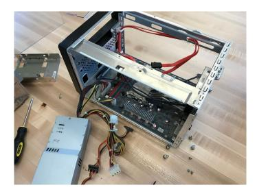
The case serves many important functions. It keeps dust out, cools the entire system with fans, and houses the main controls like the power button.
