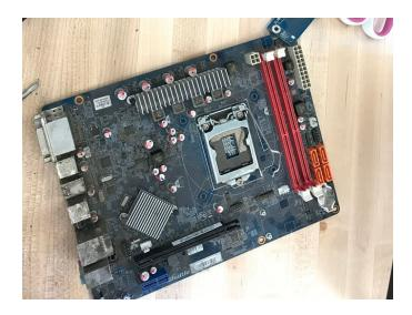
A top down view of the motherboard shows some key features. The red slots are memory slots, and the CPU slot is in the center.
