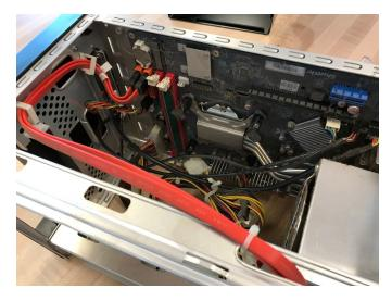
Here is a top view of the shuttle desktop. Red cables are the SATA cables that connect storage devices to the motherboard.
