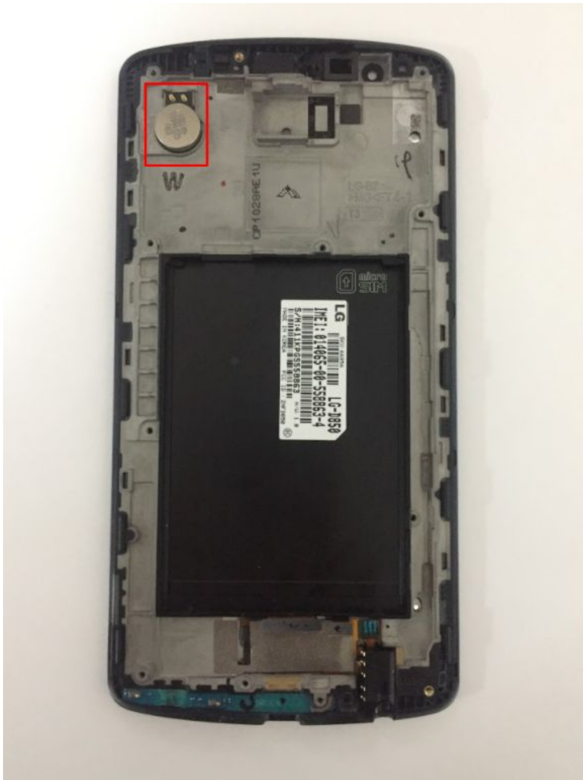
This is the phone case with the motherboard and other components removed. The piece which is boxed in red is the LG G3 Vibrator.
