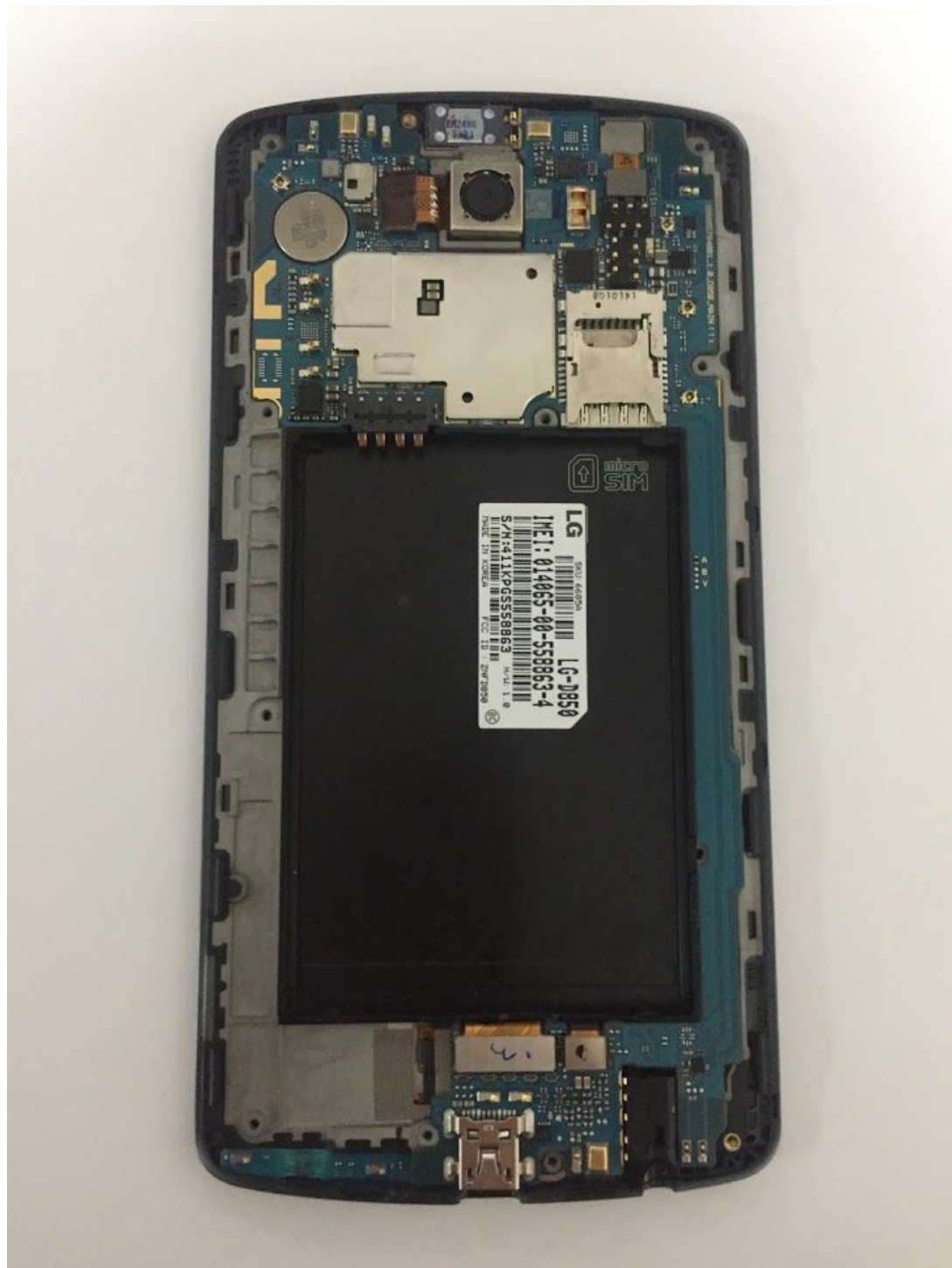
This is the LG G3 phone with the back and phone cover removed.
