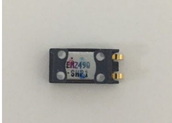
This is the LG G3 earpiece speaker which produces sound from electric impulses on a phone. (front and back)
