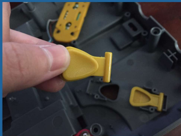
FIGURE 2.13: Yellow buttons for the different channels on the controller
