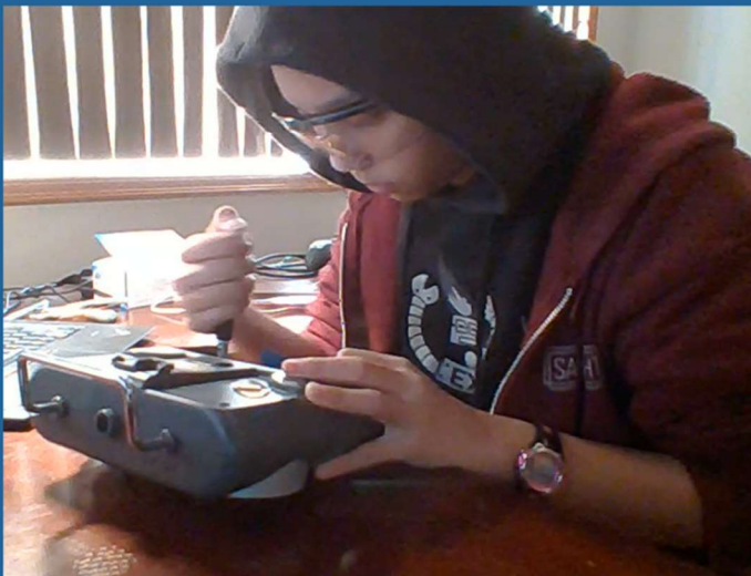
FIGURE 2.2: Removing screws on the back of the controller
