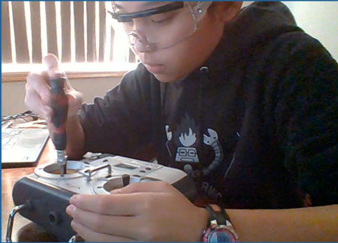
FIGURE 2.0: Removing screws on the front of the controller
