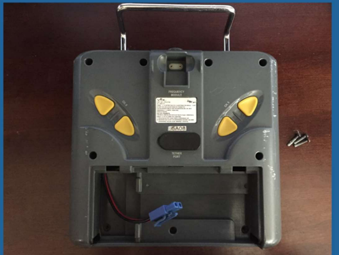
FIGURE 2.3: Three of the back screws removed
