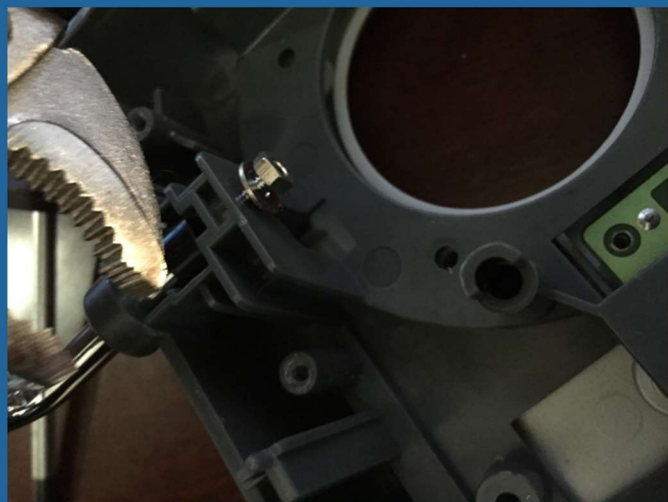
FIGURE 2.25: Loosening the nut attaching the metal handle to the case w/ pliers
