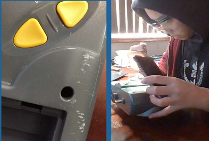
FIGURE 2.6 – 2.7: Using a phone's flashlight to examine a stripped screw
