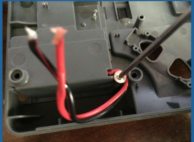
FIGURE 3.4: Freeing the battery wire from the case
