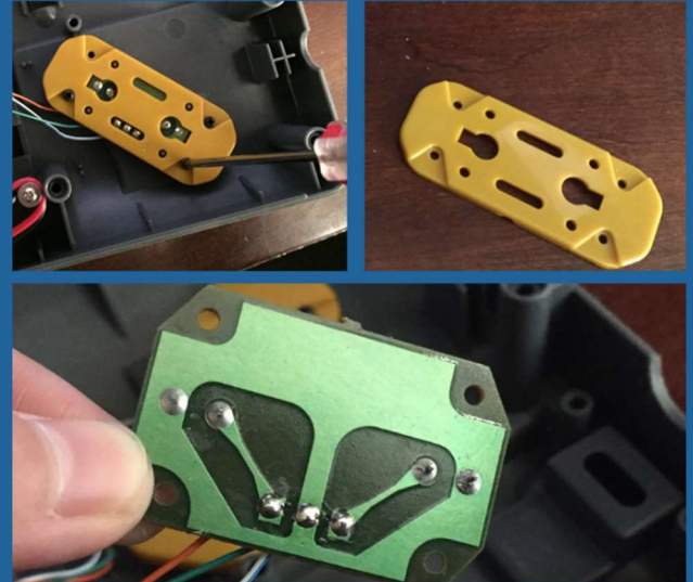
FIGURE 2.10 – 2.12: Taking off the yellow cover protecting a circuit board
