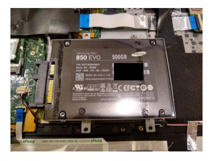
The SSD is where all of the files and applications are stored. Since SSDs utilize flash-based memory, it can achieve high read and write speeds.
