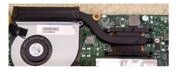
The CPU, or Central Processing Unit, is the electronic circuitry that executes instructions for a computer program. It's covered by a heatsink to keep cool.
