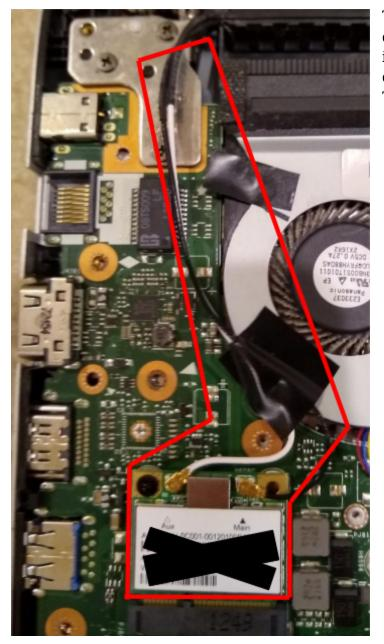
This module is responsible for connecting the computer to the internet and allowing Bluetooth connection from external devices. The screen is used as an antenna.
