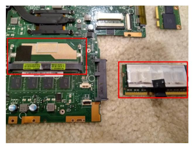
The RAM or Random Access Memory is an onboard storage device that holds short-term data for the computer while in use.
