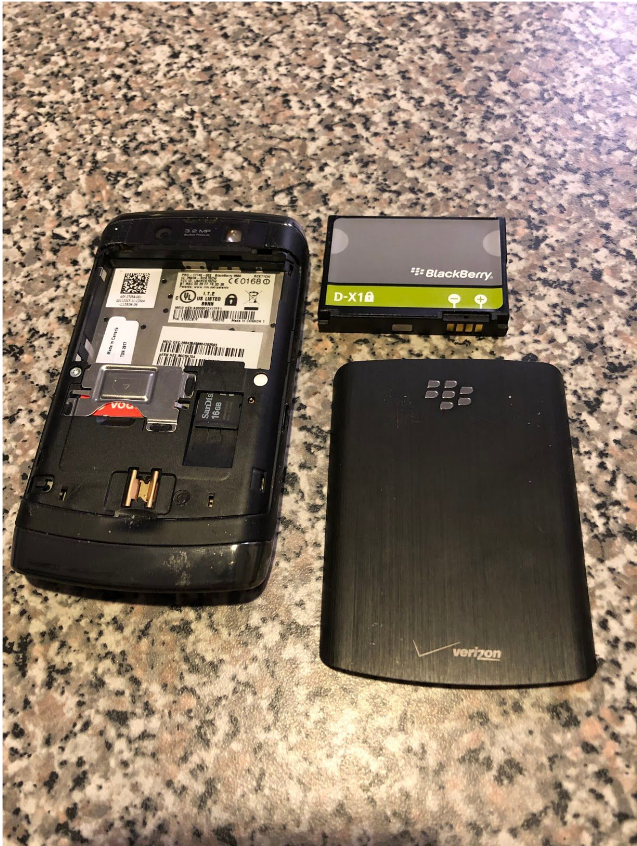
The back lid and Lithium ion battery taken out of the phone
