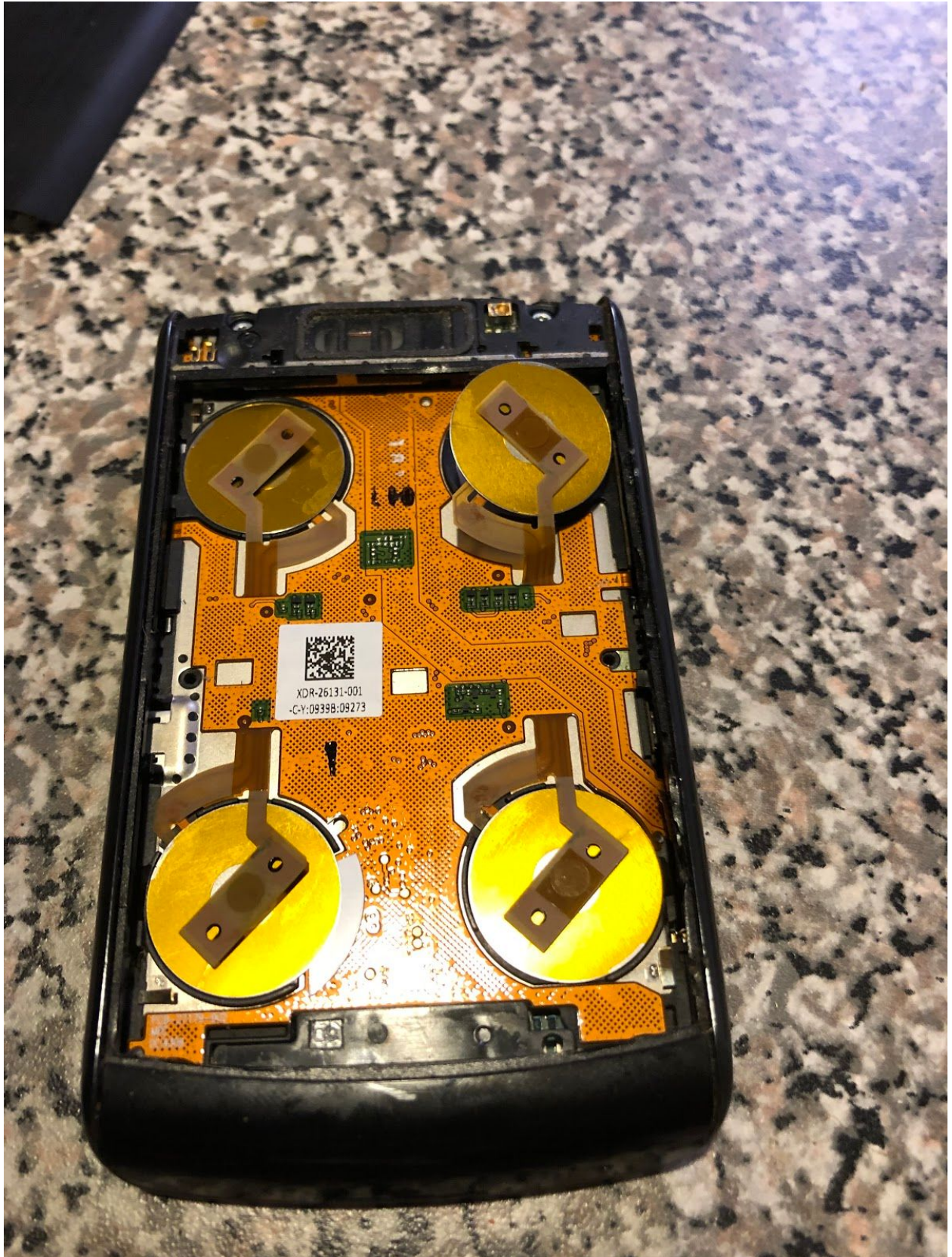
The Screendriving Circuit Board and the 4 piezoelectric discs inside the phone
