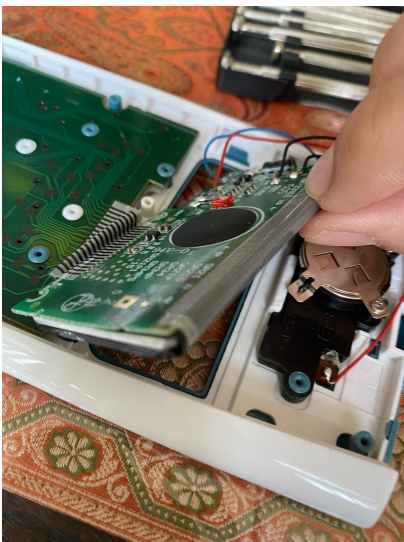
This is the display, which is an LCD, and physically displays the result of the typed buttons
