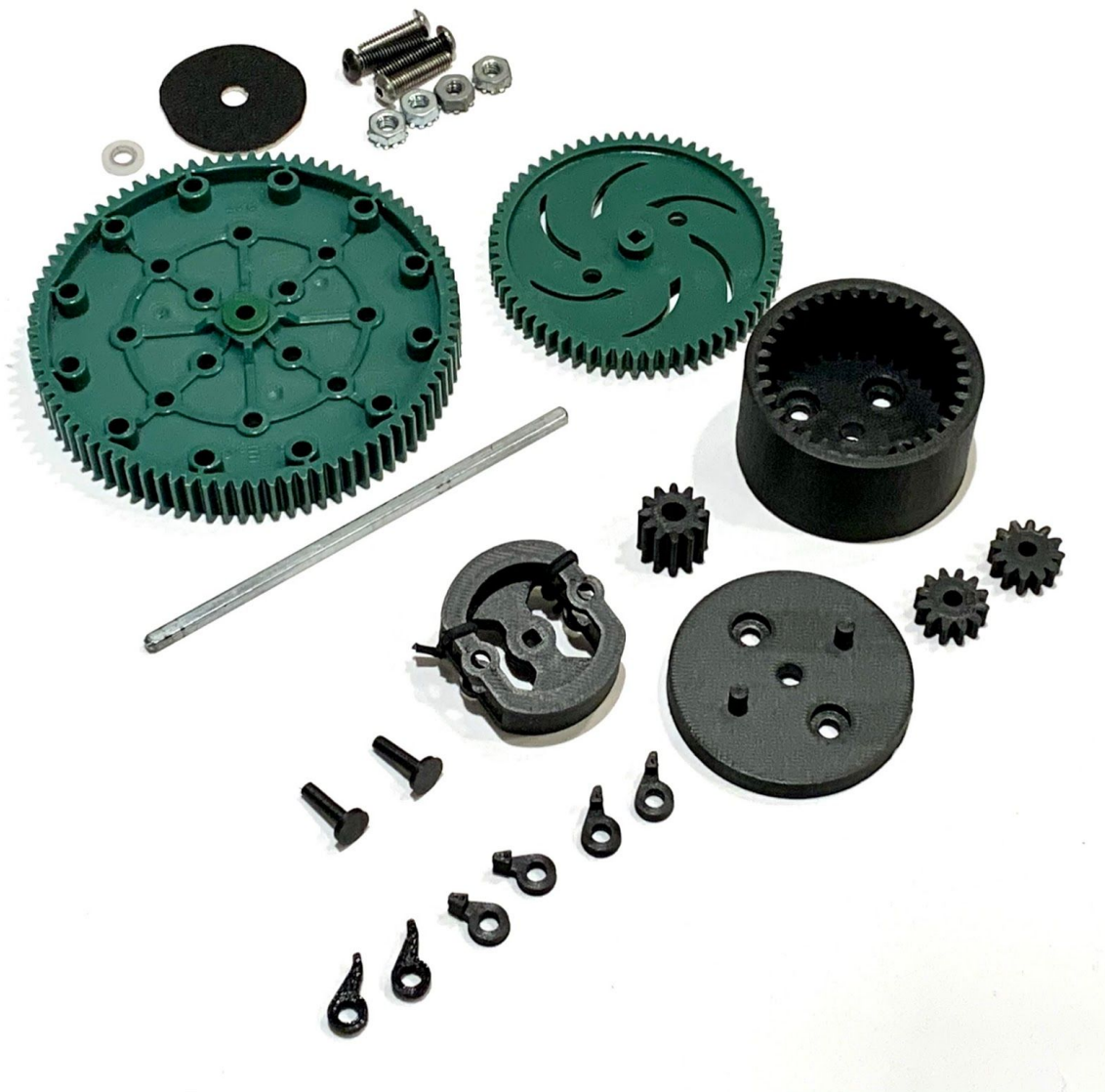
All parts used in the planetary 2-way ratchet. 3D printed parts are at the bottom, and VEX parts are at the top. There are also custom rubber bands on the inner ring and a cardboard spacer at the top.
