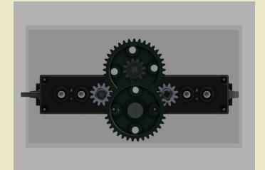
At the making progress of the transmission we used three gear wheel with twelve gear tooth, two gear wheel with thirty six gear tooth and three shafts.
