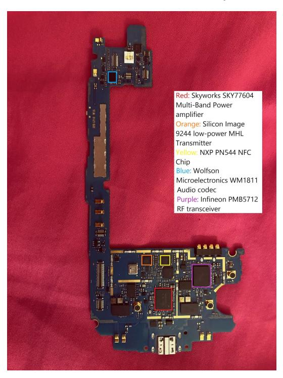
This is the bottom of the Motherboard with its labeled components.
