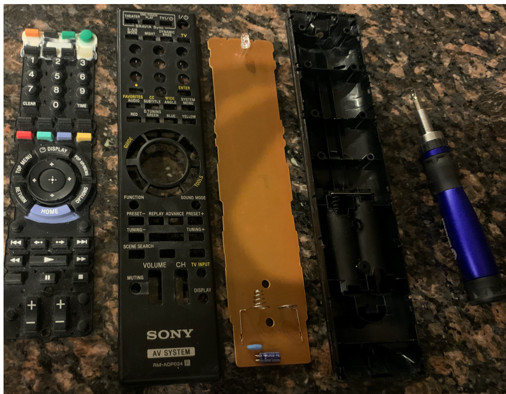
Figure 2: The components of the remote after being disassembled
