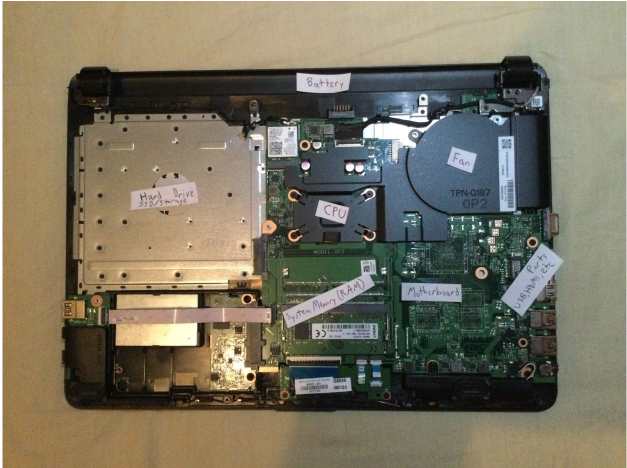
After, I identified and labeled all of the parts included inside the laptop. Then, I made some research in order to fully understand these components.
