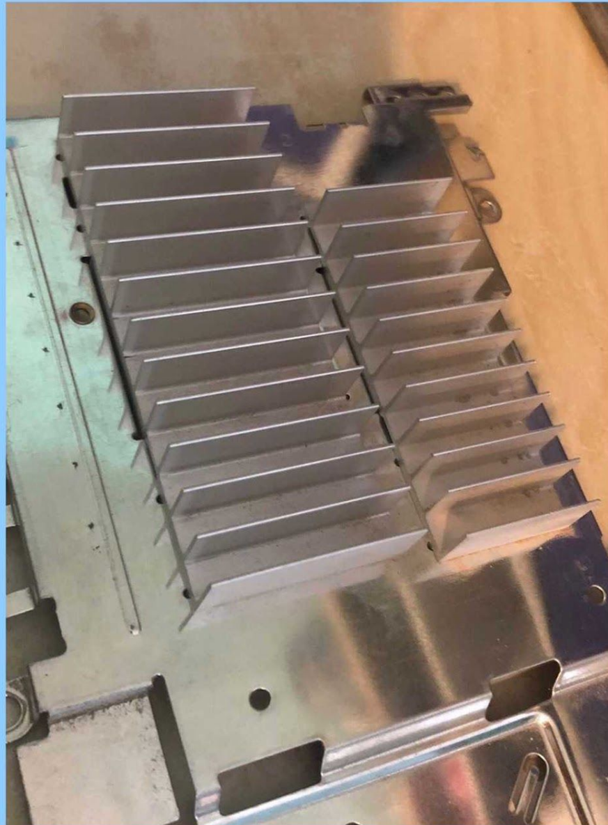
The heat sink that directs heat away from the motherboard
