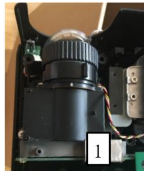
Figure 7: Projector Lens. 1 - DMD Chip and Holder, which are right behind the projector lens.
