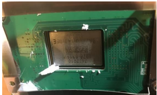
Figure 5: Metal traces on back of DMD chip
