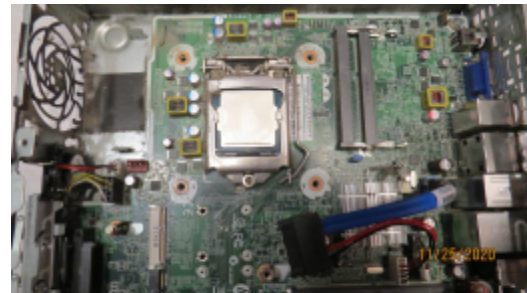
Processor in the LGA1155 socket in the motherboard prior to being taken out for analysis.
