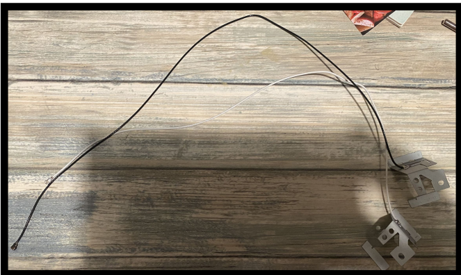
Figure 6. The antennas are two thin wires.
