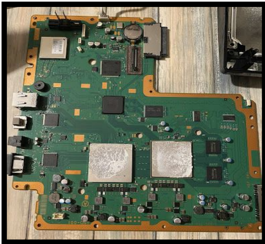
Figure 1: This is the motherboard of the PS3.
