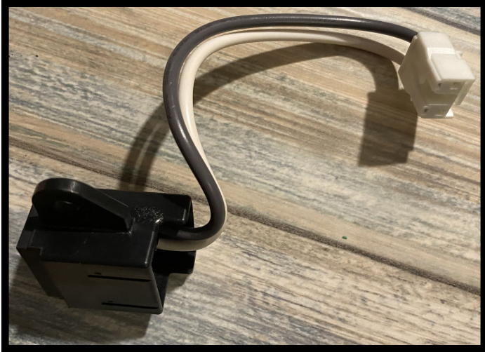
Figure 4: This wire is the AC Inlet.
