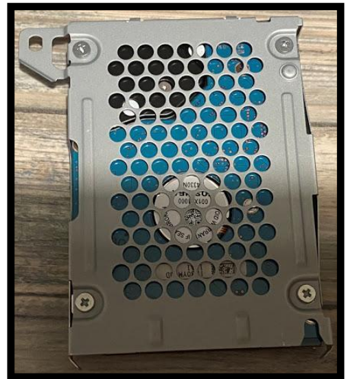
Figure 5: This is the picture of the hard drive in its casing in the PS3.
