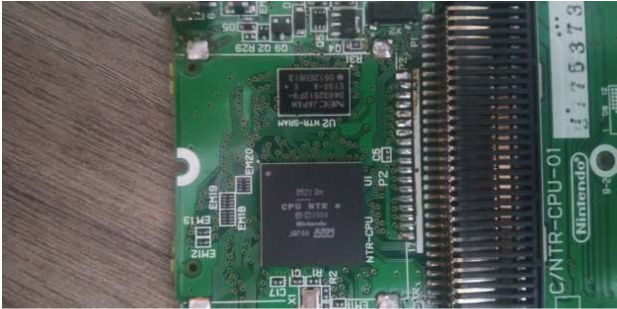
Figure 2 - The NTR-CPU and 4K PSRAM underneath the Game Card slot.
