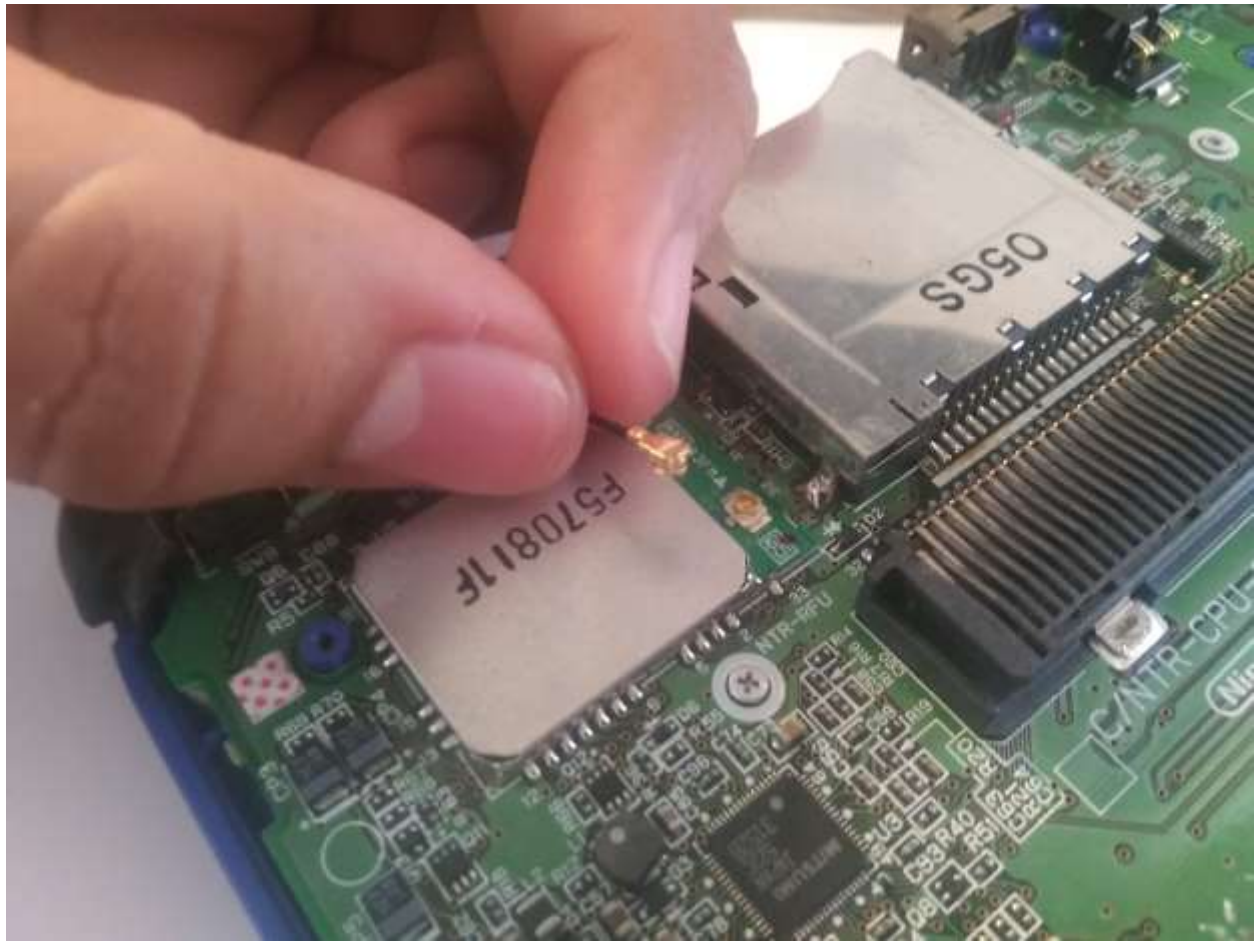
Figure 7 - Disconnecting the cable for the Mitsumi WiFi Adapter.
