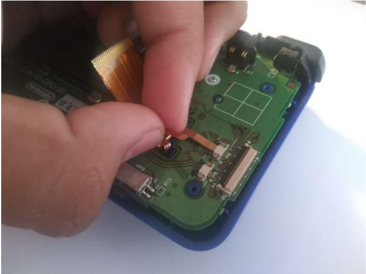
Figure 6 - The cables used for the screen digitizer and bottom TFT screen.
