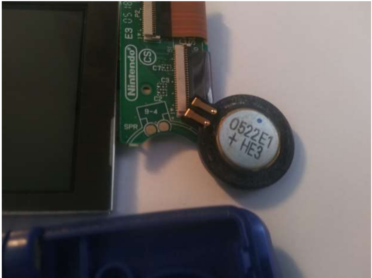
Figure 8 - A daughterboard used to connect both screens and the right speaker.
