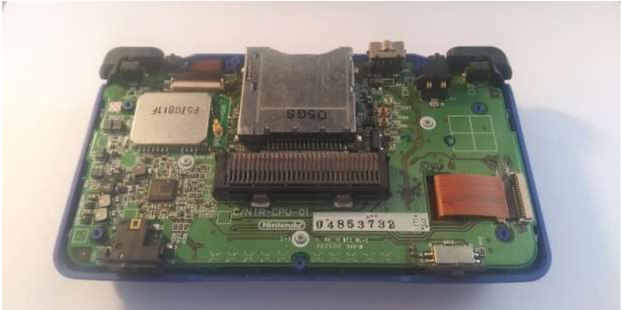
Figure 5 - The Nintendo DS motherboard after removing the back cover.
