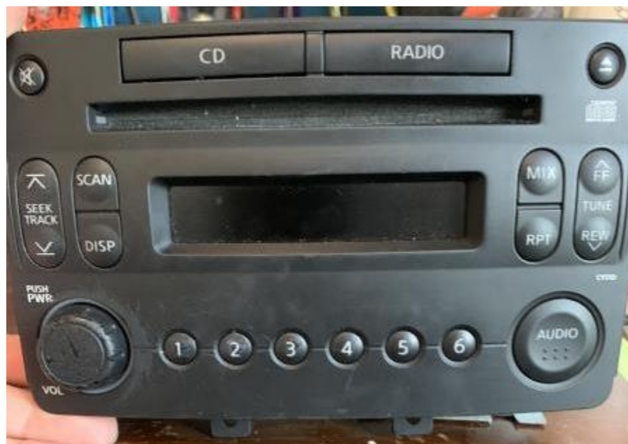
Stock Nissan 350Z 2008 Stereo - A small stereo unit used in various vehicles. It features a CD drive, radio, and LCD.
