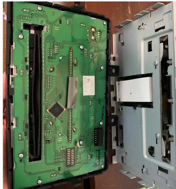
Top View of the front panel PCB
