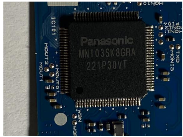
Panasonic Chip Model #MN103SK8GRA. It communicates with the laser.
