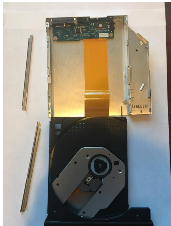
This is the disk drive with the cover of. We had to remove the rails because the disk drive was not powered. At the top of the picture the interfacing board.
