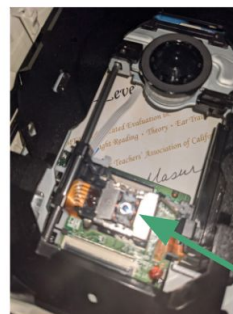
The laser reader starts shining light on the disk, however, when the light hits a bump, the reflection is different to when there's no bump.
