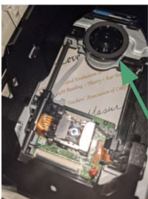
The CD goes into a slot where it is read. When you start the disk drive, the disk drive motor starts spinning the CD.
