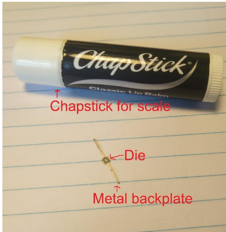
Figure 6. A photograph of the retrieved die mounted on its metal plate with a Chapstick for scale.
