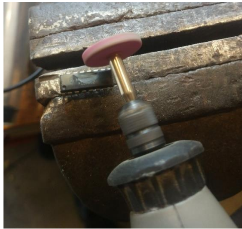
Figure 2. As much plastic as possible was removed with a Dremel tool, reducing the amount to be slowly dissolved. Safety equipment was worn.
