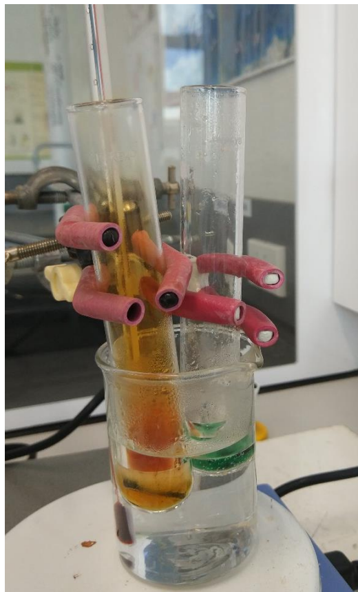
Figure 4. An early attempt. Note the red nitrogen dioxide fumes from the copper wires reacting with the nitric acid.
