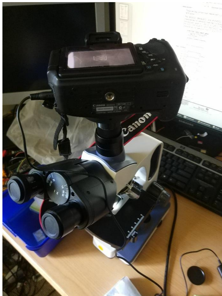
Figure 7. The microscope and camera used to photograph the die. The following die photos were taken at 100x zoom
