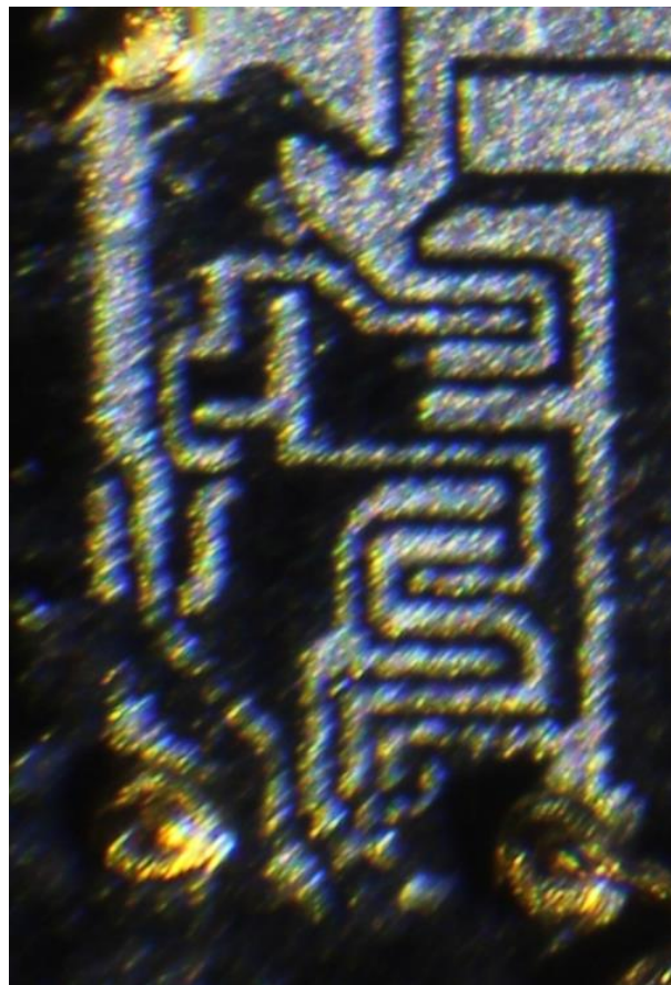
Figure 14. A closeup of 1 gate. Transistors can be identified by a cluster of 3 nearby parallel wires – for base, collector, and emitter.
