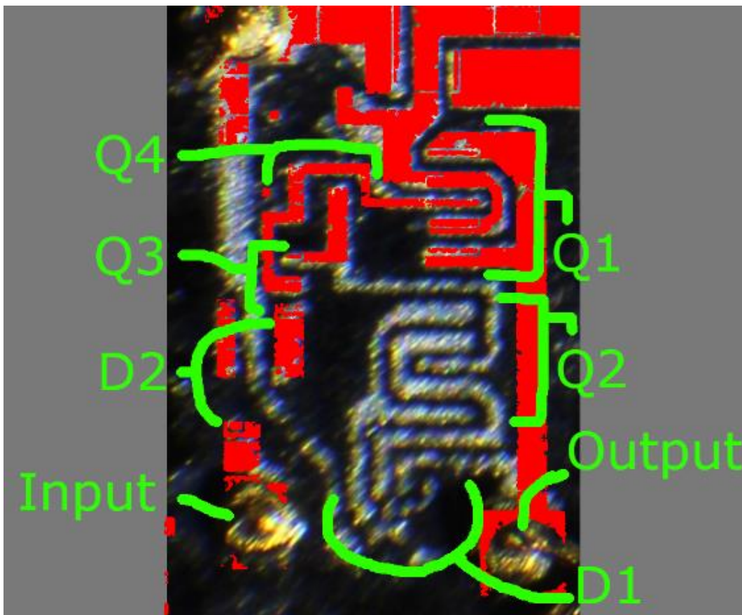
Figure 16. Red overlay is SN7405 with 1 less transistor and diode than SN7404, helping us to estimate components. D = diode, Q = transistor
