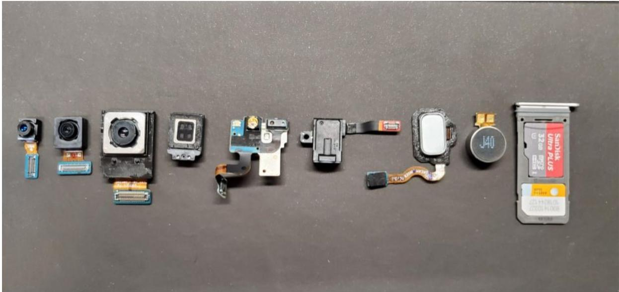
These are the various components of the phone that were removable from the boards that control the majority of the functions.
