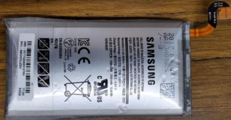
This is the lithium ion battery that was found inside of the phone. It has expanded from being placed in an improper environment.
