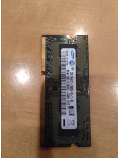
This is the RAM (Random Access Memory) of the HP mini laptop 5103.
