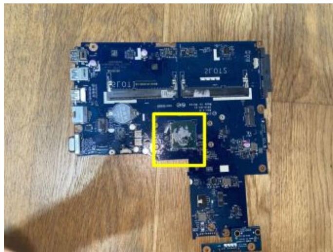
Motherboard found inside & the CPU is highlighted in the yellow box
