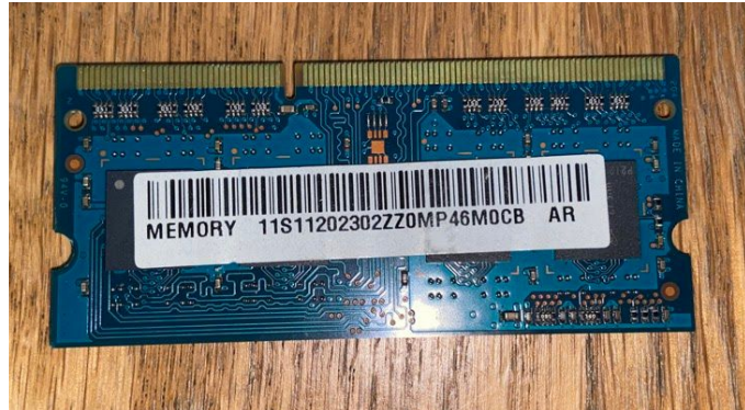
The RAM Component found in the device: RAMAXEL 4GB RAM
