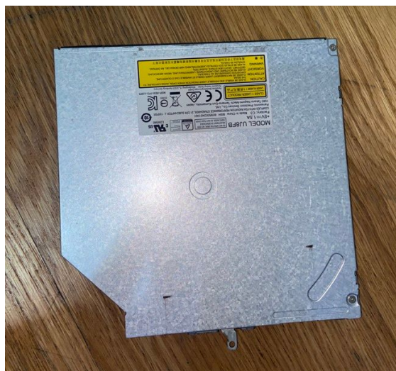
Panasonic UJ8FB 9.5mm Sata Internal Slim DL DVD CD RW Burner Drive
