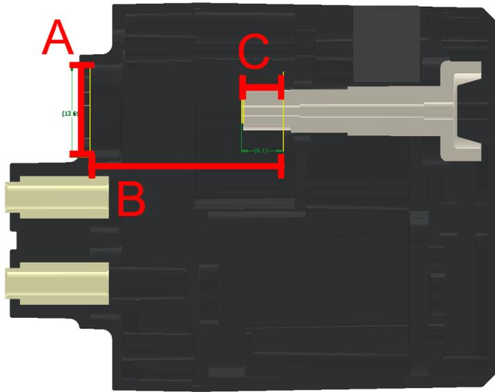
In order to design this part, we utilized the CAD files of a V5 motor made available on the VEX Robotics website. After it was imported into Autodesk Inventor Professional 2021 we deleted the cartridge that came inside the motor and made a sketch of the pertinent project geometry. Then, we copied this sketch into a new parts file. We found measurements inside the motor which allowed us
