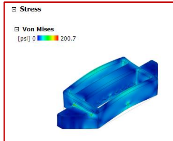
Fig 11. Static stress demonstrates how the modular wheel bay will deform under load.
